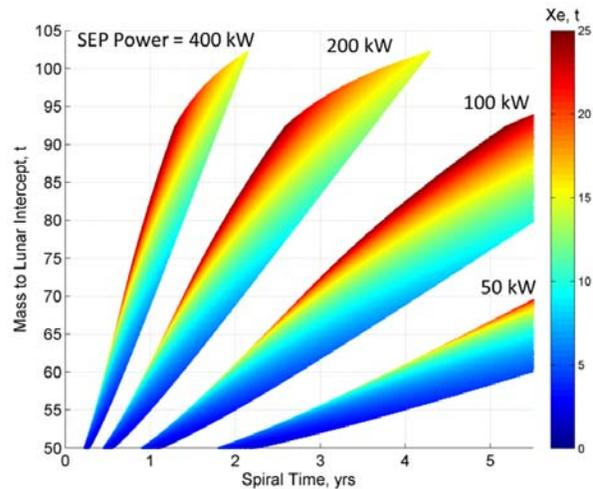
**Figure 1.** SEP can roughly double the mass delivered to lunar-crossing HEO from a single SLS launch. The specific SLS assumptions to recreate this figure are 241 km LEO, 140.8 t in LEO with 23.6 t inert upper stage, 462 s  $I_{sp}$ . SEP spiral to 384000 km circular orbit for Lunar intercept, 44% efficiency at 1500 s, 67% efficiency at 5000 s.
