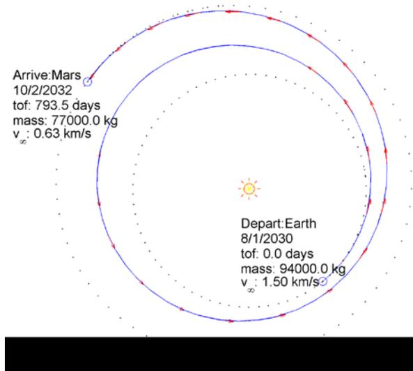
**Figure 2.** A 270-kW SEP vehicle can perform a 1.5-revolution transfer to Mars (preceded by a geocentric spiral and lunar-assisted escape) and combined with a high-thrust capture maneuver at Mars would deliver a 70 t of payload to a 1-sol orbit from a single SLS Block 2 launch.
